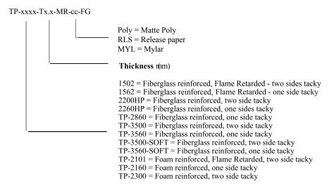
Standard Packaging Thin Fiberglass Reinforced Thermal Gap Pads
